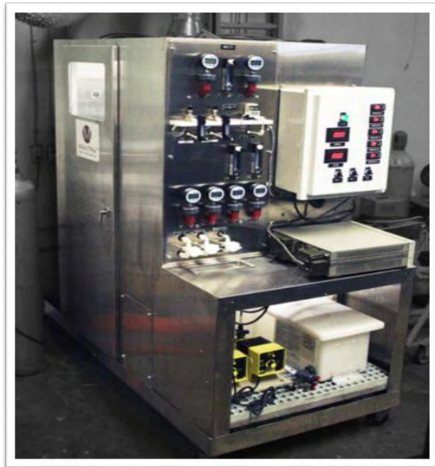
Pilot-scale: 100 kg/day CO 2 to formate/formic acid
